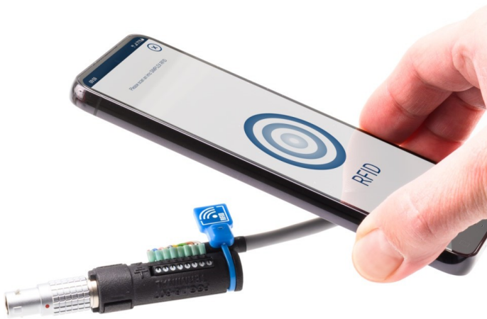
Scan sensor via cell phone
