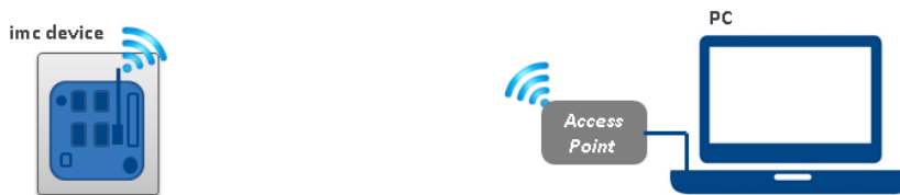
PC via Access Point - Device via integrated WLAN
